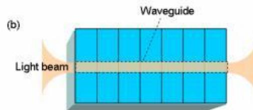
The light beam is confined in the waveguide chip.
