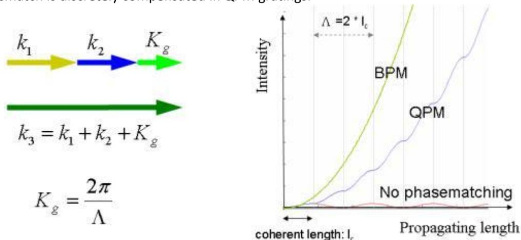
QPM structures are most commonly obtained by periodic poling of ferroelectric crystals like lithium niobate (LiNbO<sub>3</sub>) and lithium tantalate (LiTaO<sub>3</sub>). The most widely used method for periodic poling makes use of electric fields. The principle is that the spontaneous polarization in a ferroelectric material such as lithium niobate can be reversed periodically under the influence of a sufficiently large electric field (In general, it is meant to be "periodically poled").
